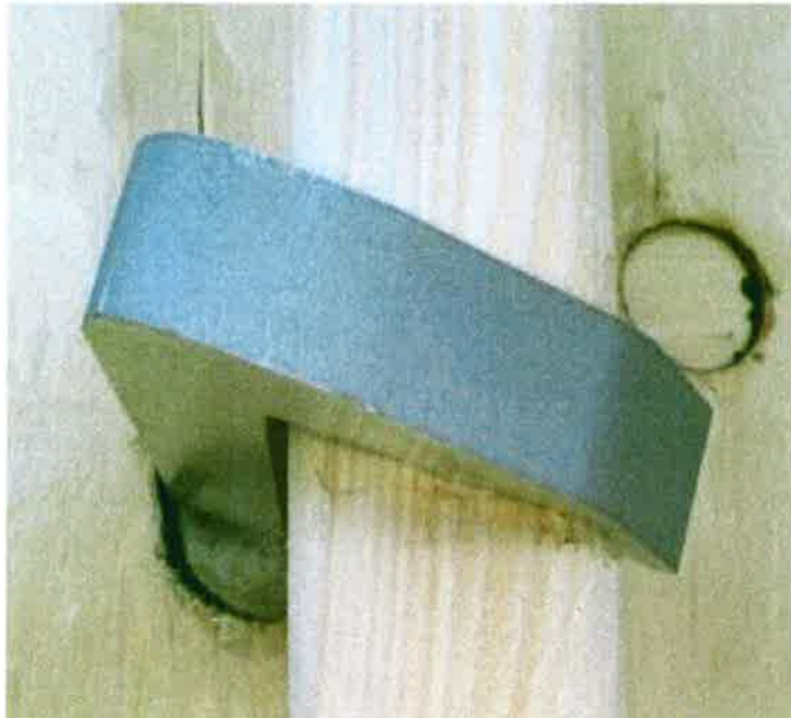
Photo 2: “J-hook” after load test.
